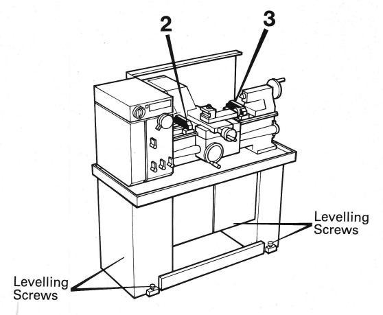
Boxford part numbered X10/14/011, or at least  $60 \times 50 \times 6$ mm  $(2\frac{1}{2} \times 2 \times \frac{1}{4})$  should be provided under each levelling screw to spread the point load and prevent the screw from digging into the floor.
